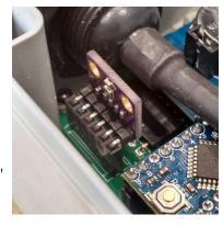
Two of these 3-in-1 sensors are used for the TrogloAir module, one is placed inside the
