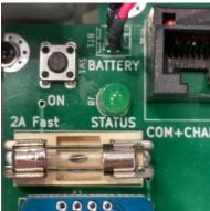
In case the user enters the boot menu, the on-board LED will flash **twice every second** for 30 seconds, waiting for the user to enter a command. If the user does not enter the boot menu or after device exits the boot menu, the device will begin to record data from the sensors. From that time on, the on-board LED will flash **once every 10 seconds** while in data-logging mode, indicating normal operation.
